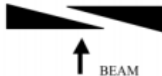
Figure 7: Dynamic X-ray beam attenuator used for maintaining constant the output photon energy while the input energy is decaying [18]
